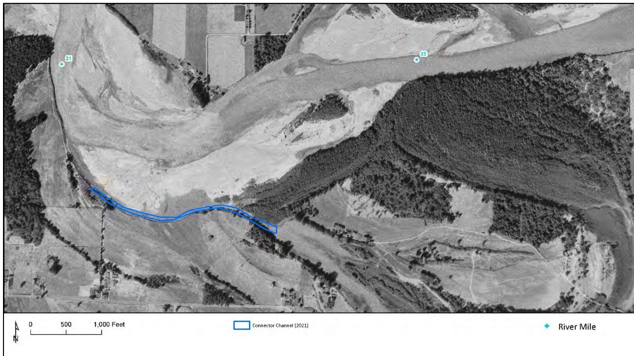
Figure 23. 1951 aerial imagery of the project area compared to the 2021 location of the connector channel. The connector channel appears to have formed along the left bank of a former Skagit River main-stem channel and has remained relatively stable since its formation after 1951.
